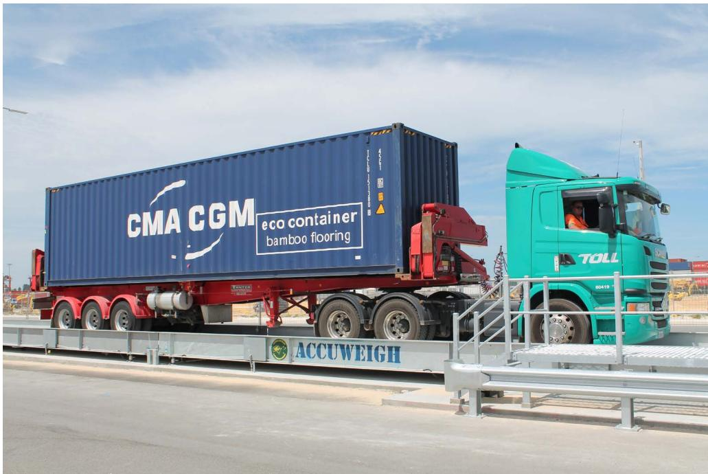
Truck weighbridge at North Quay, Port of Fremantle. Photo courtesy of Fremantle Ports.
