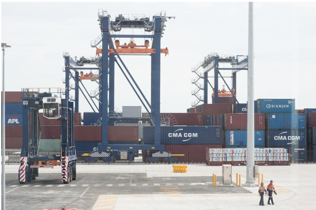
Automated Stacking Cranes tower over Brisbane Container Terminal employees. BCT was the first to introduce the Automated Stacking Systems into Australia. – photo courtesy of Hutchison Ports Australia.
