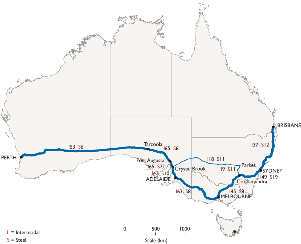
Figure 22 Number of interstate intermodal and steel trains per week on interstate track, by line segment, June 2010
