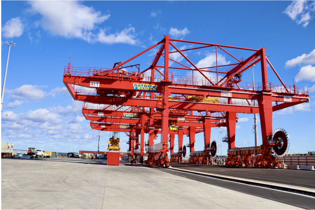
Commissioning of automated rail mounted gantry (ARMG) cranes at the new Patrick Sydney AutoRail Terminal, June 2020. Photo courtesy of NSW Ports.
