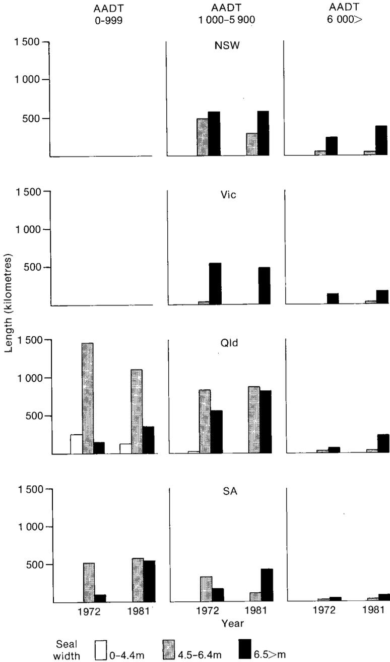
Figure 2.8—Length of seal width by AADT distribution for rural arterial roads, 1972 and 1981
